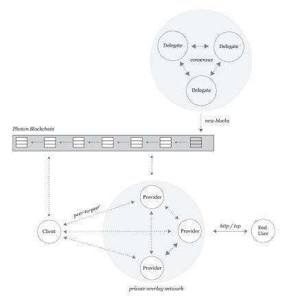
Figure 1: Illustration of on-chain and off-chain interactions amongst various participants in the Akash network
