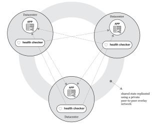
Figure 3: Illustration of Akash's overlay network
