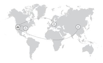
Figure 4: Illustration of slower performance due to higher latencies for endusers distributed across the globe for a single datacenter deployment
