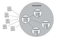
Figure 7: A machine learning batch job under load running a single master and multiple worker nodes
